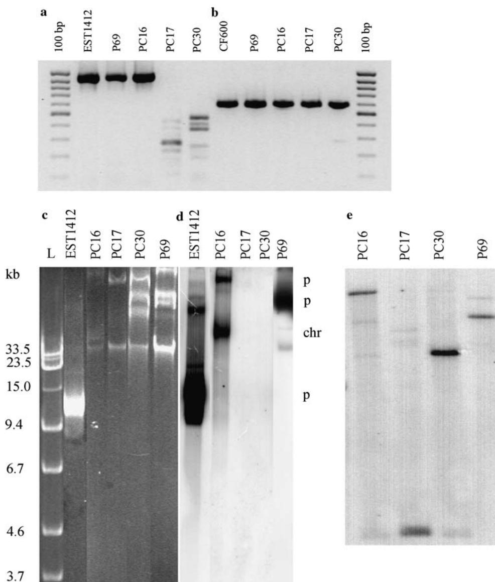
**Fig. 2** Agarose gel electrophoresis of *pheA* (a) and LmPH (b) gene fragments amplified from the *pheA*<sup>+</sup> reference strain *P. putida* EST1412, the LmPH<sup>+</sup> strain *Pseudomonas* sp. CF600 and the strains P69, PC16, PC17 and PC30. Plasmids retrieved from the *pheBA* operon possessing strains P69, PC16, PC17, PC30 and the positive control EST1412 (c) and Southern hybridi-
